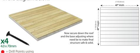
Secure roof panels by screwing them down to kennel framework as shown. Drill downwards in to the roof framwewrok so the screw meets the front & back panel framework tops. DRILL
