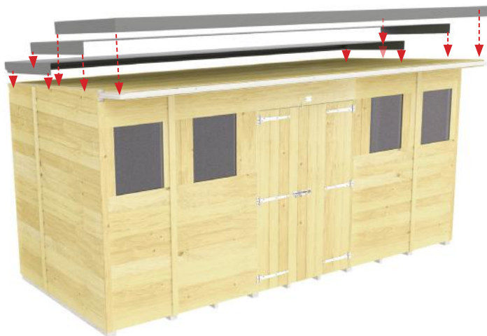
Neaten & cut excess felt
