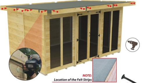
= Drill Points using screws provided as shown **18c.** Felt Strips must be same height as roofing felt to allow rain water to run off. See Diagram on the right.
