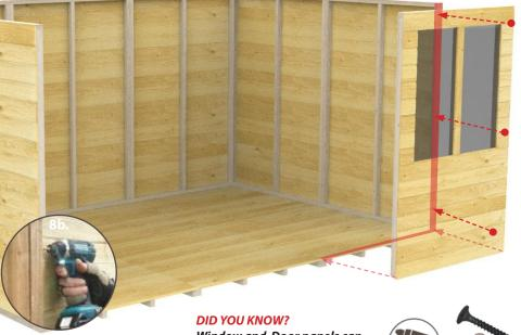
= Drill Points using screws provided as shown Window and Door panels can be substituded for a side panel of the same size.
