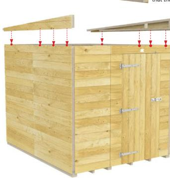
10b. Once the Pent Angle **Top** has been constructed, use the screws to secure the **Angle Tops** to the sides of the Shed.
