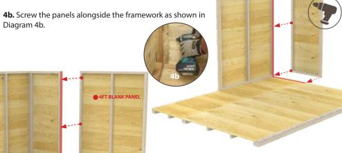
**4c.** Place the 4ft **Blank Panel** as shown along the side of the shed floor aligning with the edge of the side Floor Block. **REPEAT** this step until all back Blank Panels are in place.
