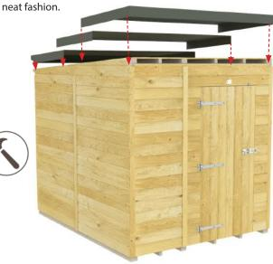
**15c.** Trim down excess felt with a stanley knife. Remember to overlay the 1st felt to avoid rain leaks.
