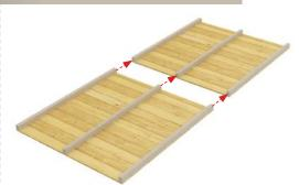
This process will be the same for any build this has a depth of 8ft. The 8ft will be constructed using two 4ft sections.
