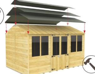
15c. Trim down excess felt with a stanley knife. Remember to overlay the 1st felt to avoid rain leaks.
