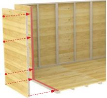
= Drill Points using screws provided as shown
