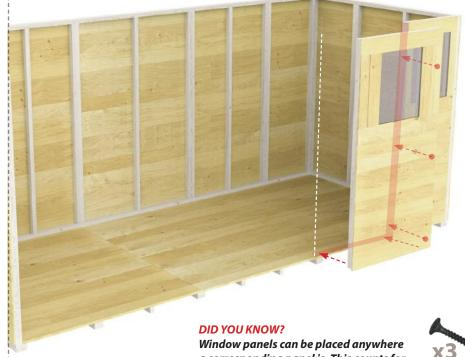
Window panels can be placed anywhere a corresponding panel is. This counts for the door panel also.
