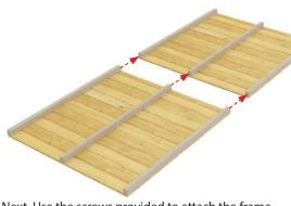
This process will be the same for any build this has a depth of 7ft. The 7ft will be constructed using one 4ft section and a 3ft section.
