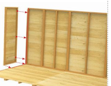
= Drill Points using screws provided as shown **DO NOT screw the standing panels** down to the floor just yet. Leave room for adjustments when the final frame is fitted.
