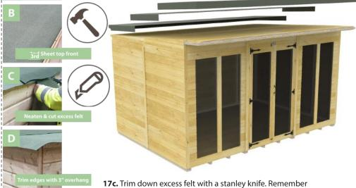
**17c.** Trim down excess felt with a stanley knife. Remembe to overlay the 1st felt to avoid rain leaks.
