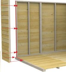
**7c.** Repeat the previous step until the walls of the shed are complete.
