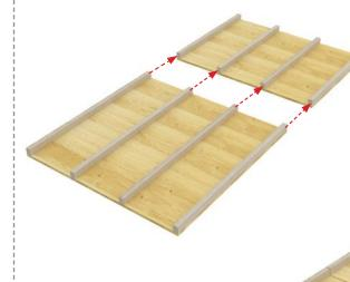
This process will be the same for any build this has a depth of 7ft. The 7ft will be constructed using one 4ft section and a 3ft section.
