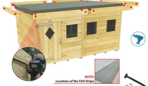
**16c.** Felt Strips must be same height as roofing felt to allow rain water to run off. See Diagram on the right.
