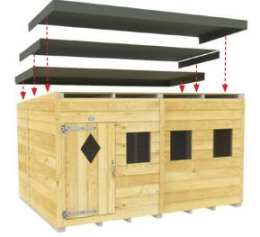
**15c.** Trim down excess felt with a stanley knife. Remember to overlay the 1st felt to avoid rain leaks.
