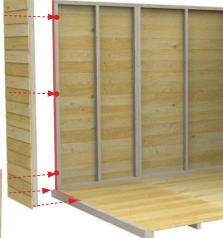
**7c.** Repeat the previous step until the walls of the shed are complete.
