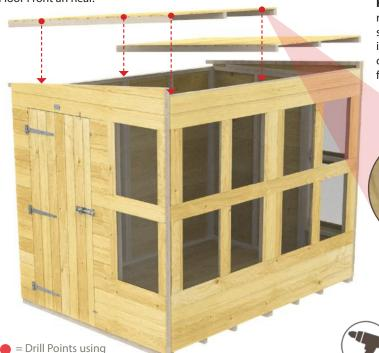
**Repeat** this for all roof panels, making sure each panel is sitting on its corresponding sized front/back panel.
