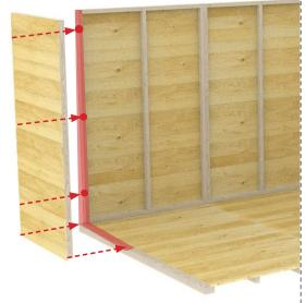
**7b.** Repeat this step until all **Side Panels** have been secured in place using three screws.
