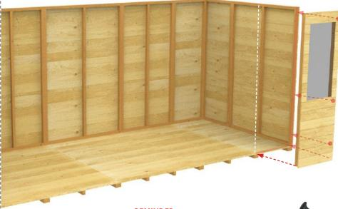
= Drill Points using screws provided as shown REMINDER
