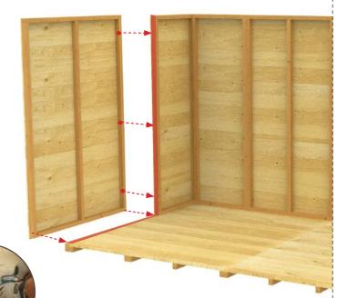
DO NOT screw the standing panels down to the floor just yet. Leave room for adjustments when the final screws provided as shown frame is fitted.
