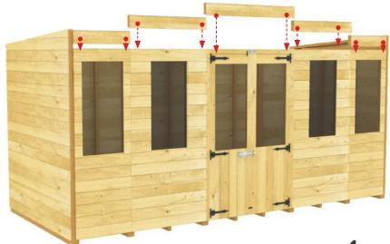
**15c.** Attach the sections down by screwing through the inner framework of both panels.
