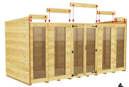
= Drill Points using screws provided as shown **15c.** Attach the sections down by screwing through the inner framework of both panels.
