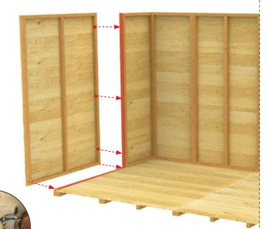
DO NOT screw the standing panels down to the floor just yet. Leave room for adjustments when the final frame is fitted.
