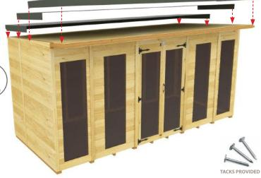
**20c.** Trim down excess felt with a stanley knife. Remember to overlay the 1st felt to avoid rain leaks.
