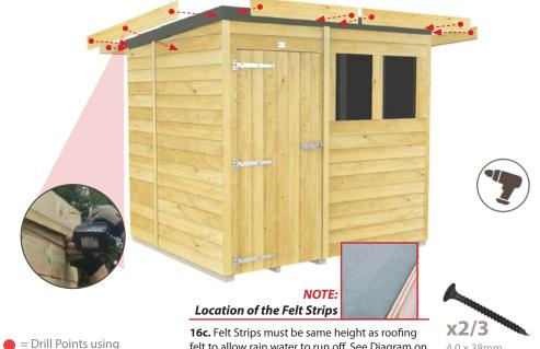
**16c.** Felt Strips must be same height as roofing felt to allow rain water to run off. See Diagram on
