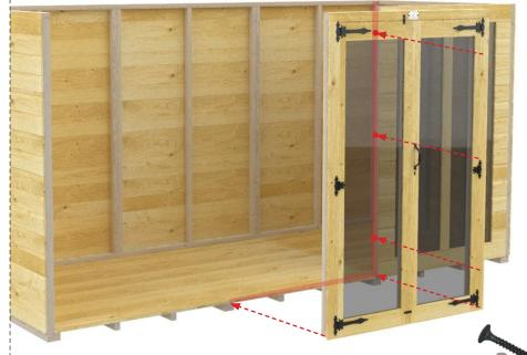
= Drill Points using screws provided as shown
