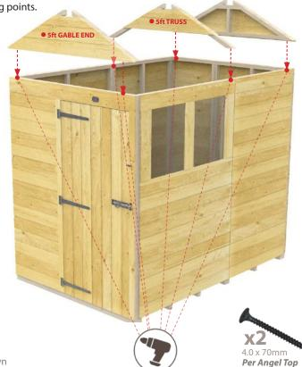
= Drill Points using screws provided as shown
