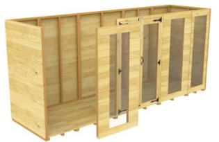
**9a.** Place the final front panel as shown (Below) to complete the outer framework. Then adjust and screw down the panels to the shed floor to make the build secure. This requires an extra 3x Screws.
