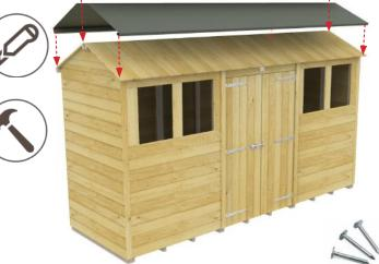
**13c.** Trim down excess felt with a stanley knife. Remember to overlay the 1st felt to avoid rain leaks.
